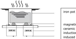
magnetic circuit ceramic glass plate induction coil induced currents
