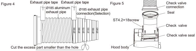
Note: During installation, straighten the aluminum exhaust pipe to avoid noises in semi-stretched state.Excess part may be cut with a wire cutter.
