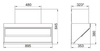
The marked sizes are for reference only, the depth dimension includes machine feet. (Unit: mm) Note: If the hood is to be wrapped into the cabinet, the inside dimensions of the cabinet should be larger than the dimensions with \*.323mm is the depth without the main panel, and 328mm with the main panel.
