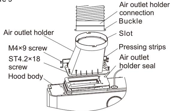
Note: Please install the air outlet seat seal with the adhesive side facing up.
