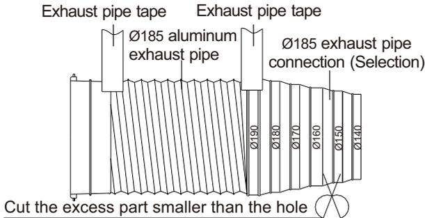
Note: During installation, straighten the aluminum exhaust pipe to avoid noises in semi-stretched state. Excess part may be cut with a wire cutter.
