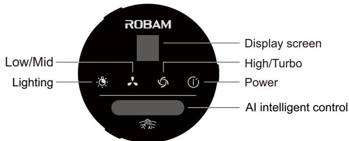
Turn on the power, the buzzer sounds to indicate the power-on state.
